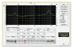
In addition to note-by-note voicing, Allen's DOVE<sup>TM</sup> voicing software offers parametric equalization and other exclusive capabilities to assist the voicer in tailoring the sound of the organ to the room's natural acoustic.
