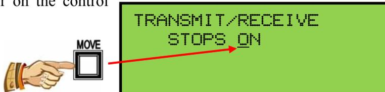
Turn the **CHANGE** control knob to change the transmit/receive status on or off.
