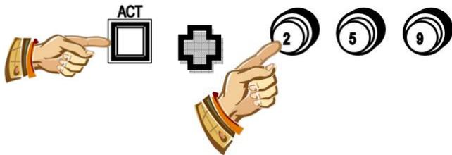
lock this memory (See Section A-5). Release the **ACT** button. If the correct code is entered, the "L" will disappear, indicating the selected memory is now unlocked.
