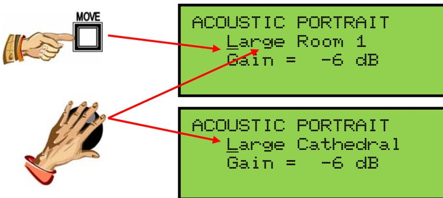
**Note:** The selection change will not be immediate. The newly selected Acoustic Portrait pallet will begin loading in approximately 3 seconds. The display will indicate the newly selected pallet is loading and when it has completed:
