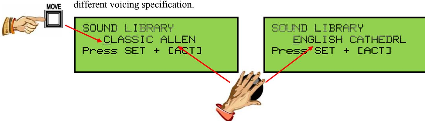
When a new voicing specification is displayed, press and hold the **SET** piston. Then, while holding **SET**, press the **ACT** button. Release both.
