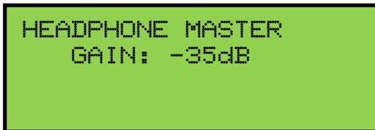
To change the Headphone Master Gain setting, press the **MOVE** button to position the cursor on the Gain setting value. Turn the **CHANGE** control knob to change the gain setting. Gain adjustment range is from (off) or minus 35dB to 6db. Minus 35db is the least amount of gain while 6db is the most or maximum amount of gain.
