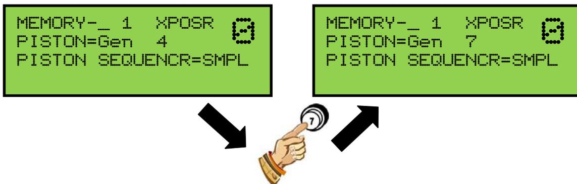
The capture memory level may also be changed at any time while within SIMPLE STEPPER mode. To change the capture memory level, press the **MOVE** button to position the cursor on capture memory level value. Then, turn the **CHANGE** control knob to select a different capture memory level (*see Section A-3*).
