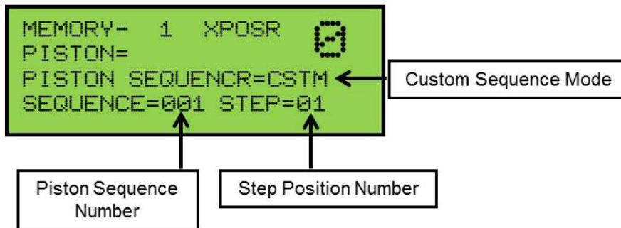
From here, the organist can select a custom piston sequence to use and step position. The capture memory level and piston display will reflect the programmed data within the selected step position number.
