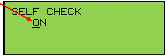
During the testing process you can stop the Self Check function at any time by turning the **CHANGE** control knob until "OFF" appears within the display or by using the **SET** and **CANCEL** pistons to also return to the *Main Window* function (*see Section A-2*).
