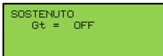
The display will indicate which manual *Sostenuto* is assigned to and indicate the current on/off status.
