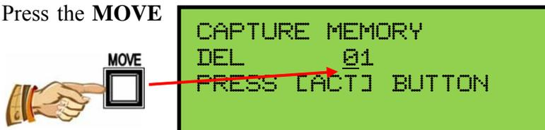
Turn the **CHANGE** control knob to select a capture file number. Turning the knob clockwise will increase the file number while turning the knob counter-clockwise will decrease the file number. Any file number between 01 and 99 may be selected.
