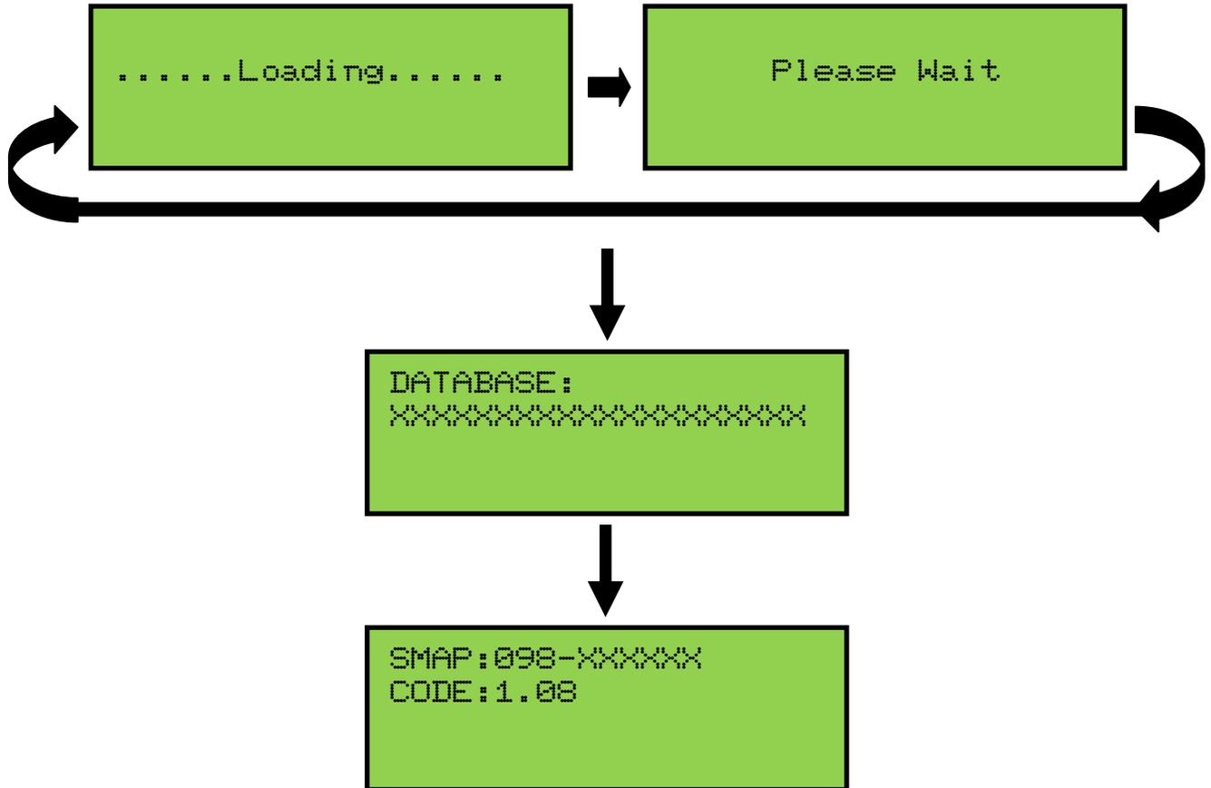
Once the GeniSys™ computer has completed its initial start-up procedure, the LCD will display the current stopmap level (SMAP) and operating software base code level (CODE) currently installed in the organ.
