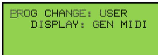
Advance to the next window function then press a piston to view the sound names for any General MIDI device. The next window will display:
