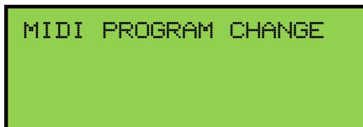
When a General piston is pressed, the GeniSys™ Controller™ will display the General MIDI sound name which corresponds to the MIDI program change selected. For example, press General Piston 1. The GeniSys™ Controller™ will display the MIDI program change name assigned to that piston.
