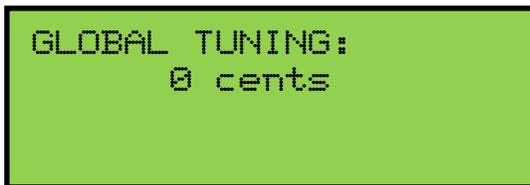
Press the **MOVE** button to position the cursor on the tuning value. Turn the **CHANGE** control knob in either direction to raise or lower the pitch of the organ. Turning the knob clockwise will raise the pitch while turning the knob counter-clockwise will lower the pitch.
