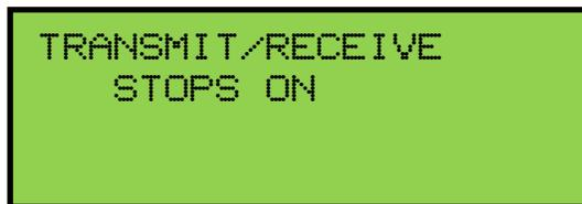
To change the on/off status of the Transmit/Receive Stops function, press the **MOVE** button to position the cursor on the control value.
