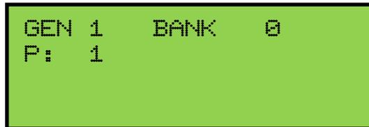
The window will display the piston pressed, the MIDI BANK Number, and the program number being sent by that piston.
