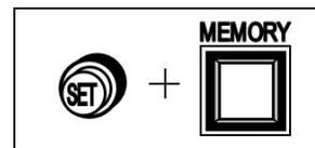
Release both the **SET** piston and **MEMORY** button. Step 1 is now programmed. Repeat the above procedure to set all available crescendo step positions.
