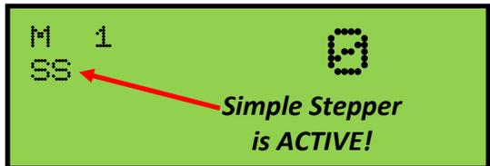
To start SIMPLE STEPPER, select a capture memory level (*see Section A-3*) and then press General piston #1. The registration associated with the selected capture memory level and General piston #1 will register on the stops and the display will indicate that General #1 has been pressed. This will also set the SIMPLE STEPPER’s starting step position.
