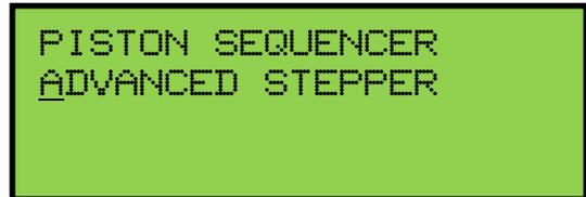
To use the ADVANCED STEPPER, return to the *Main Window* function. Press and hold the **SET** piston. Then, while holding **SET**, press the **CANCEL**.
