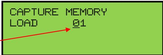
Turn the **ROTARY DIAL** to select a capture file number. Turning the Rotary Dial clockwise will increase the file number while turning the Rotary Dial counter-clockwise will decrease the file number. Any file number between 01 and 99 may be selected.
