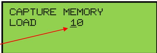
To load the selected capture file number, press the **CURSOR** button to position the cursor on the Mode value, LOAD.
