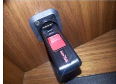
The USB flash device is used for saving or backing up the instrument's capture memories and also for the built-in Sequencer. These functions will not operate unless a USB flash device has been inserted into the USB memory port. However, the USB flash device does not need to be installed for normal playing operation of the instrument.
