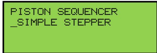
To use the SIMPLE STEPPER, return to the *Main Window* function. Press and hold the **SET** piston. Then, while holding **SET**, press the **CANCEL**.
