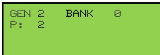
The LCD will display the piston pressed and the MIDI program number being transmitted by that piston.
