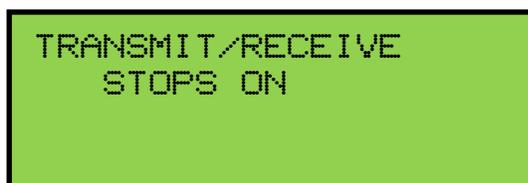
To change the on/off status of the Transmit/Receive Stops function, press the **CURSOR** button to position the cursor on the control value.
