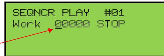
Turn the **ROTARY DIAL** to select a different counter value. Turning the Rotary Dial clockwise will increase the counter number while turning the Rotary Dial counter-clockwise will decrease the counter number.
