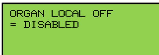
To enable/disable the Organ Local Off function, press the **CURSOR** button to position the cursor on the Local Off control value.
