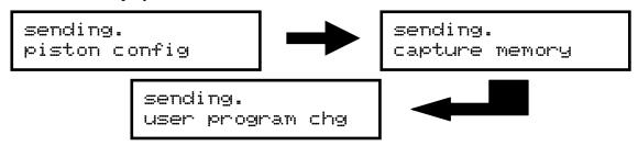
The 'dot' behind the word 'SENDING' on line one of the display will move as data is transmitted. Once the transfer is completed, the display will return to the Main window function automatically.
