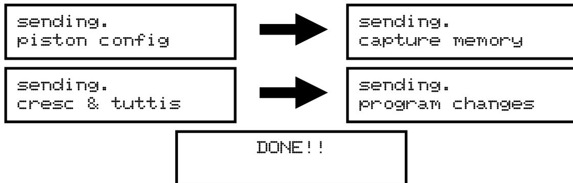
The 'dot' behind the word 'SENDING' on line one of the display will move as the data is transmitted.
