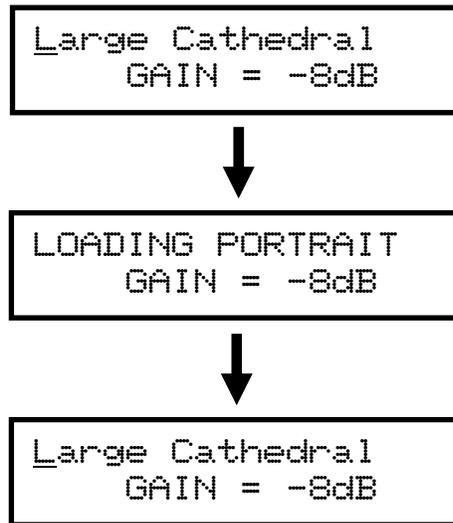
If the organ is equipped with a Quad Suite™/Stoplist Library™ Display Window, it will also flash while the new pallet is loading. Once the newly selected pallet is loaded the display will change back to the Acoustic Portrait™ pallet name and the Quad Suite™/Stoplist Library™ Display Window will stop flashing.
