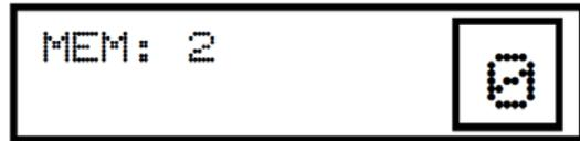
**Locking Capture Memories:** All memories, except Memory 1, may be locked or unlocked individually. While holding the “**MEM**” button, press the General Pistons to enter a three-digit code of your choice. Release the **MEMORY** button and an "L" will appear next to the MEM number in the display, indicating this memory is now locked. Use the same procedure to unlock the memory.
